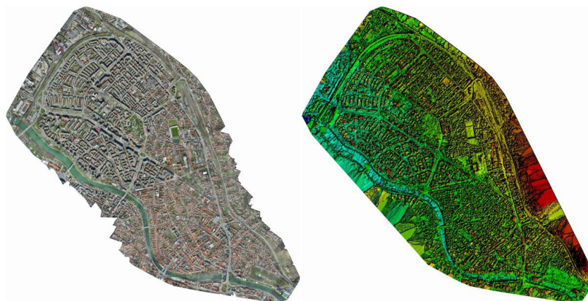
Figure 1: Orthomosaic and the corresponding sparse Digital Surface Model (DSM) before densification.
